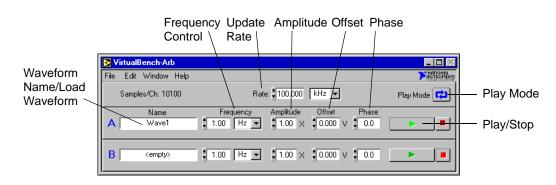
The key features of the Waveform Generator front panel of VirtualBench-Arb are:
